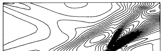
Fig. 2 Static pressure contours of the transverse He injection case.
